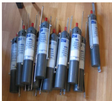
Figure 7. Location of VR2 listening stations in the Hardangerfjord in 2006. To the right is VR2 hydrophones.
